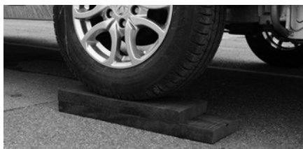
Fig. B - Levelling Board
