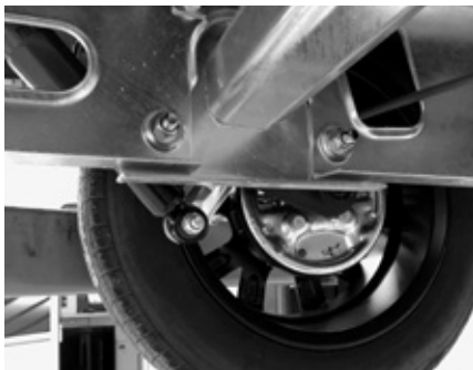
Fig. D - Reinforced axle plate
