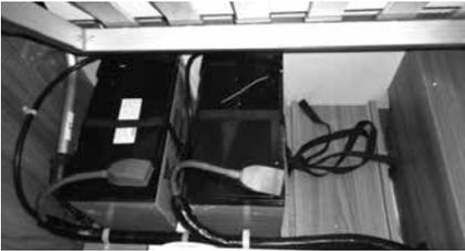
Leisure battery installation in front door side bed, showing two fitted batteries with a space for a third.
