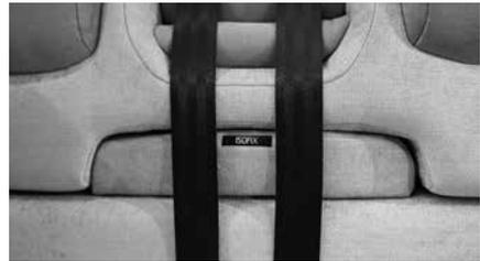
**⚠ WARNING:** Use an anti-rotation device when using the ISOFIX system. We recommend the use of a top tether position.
