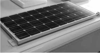
Your motorhome is fitted with a 120W solar panel and a suitable solar regulator. This solar panel and regulator may provide additional 12v power whenever sunlight is available to the panel, and this will be directed to the EC800 power supply unit. Conditions allowing, and depending on the settings chosen in the EC800 power supply unit, the system can give the leisure battery a daily boost when camping without a mains 230V supply, or while the vehicle is in storage.
