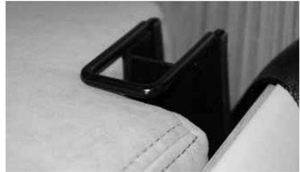
Top tether anchor points are fitted on the upper seatbelt stanchion and are accessed by removing an insert on the backrest cushion.
