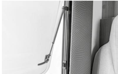
Catcher enables three positions of the window. Open position is where the handle is open placed on the outer part of the catcher. If the handle is placed in the middle of the catcher, this is position for ventilating. Closed position is position where the handle is closed on the inner part of the catcher.
