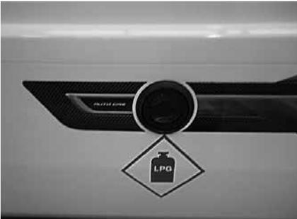
The fitting behind the cap is compatible with the filling nozzles found at UK filling stations. Adaptors are required for use with filling nozzles found in other countries.
