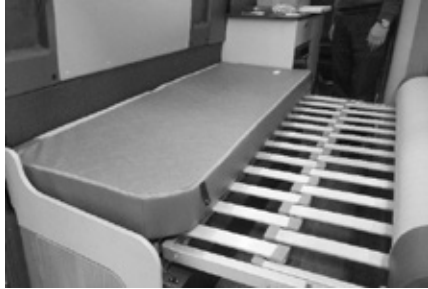
Step 7: Once the frame is located Turn the base cushions over. This creates a flat bed base.
