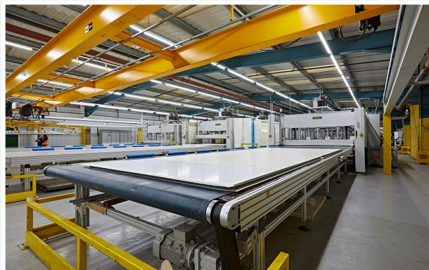
'SMART' GRP sidewall during the production process.
