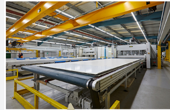
'SMART' GRP sidewall during the production process.
