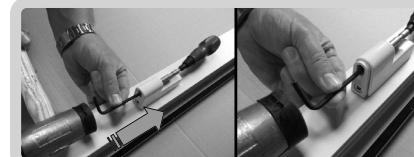
2 Insert 4mm Allen Key into hex on end of Pivot Pin
