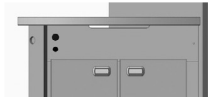
Typical 2nd thermostat and switch installation
