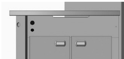
Typical 2nd thermostat and switch installation
