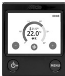
Alde controller showing fan speed selection
