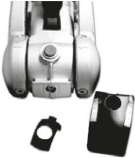
Figure 18 Cheese head screw revealed
