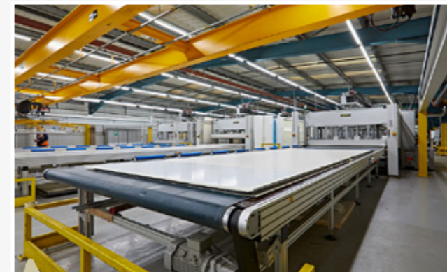
'SMART' GRP sidewall during the production process.
