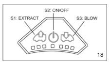
By pushing on the switch S1 (extract) or S3 (intake), the airflow can be adjusted in 6 steps. See table 19.
