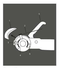
Figure 20 Friction pad revealed
