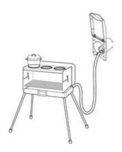
When external gas equipment is being connected, the operating pressure of the gas supply of 30 or 50 mbar must correspond with the operating pressure of he equipment that is being connected (see data plate).
