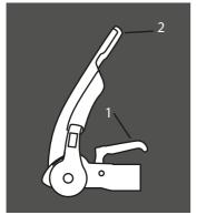
Figure 7 - Raise stabiliser lever
