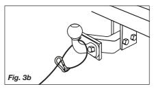
In some instances it may be possible to attach the cable assembly either to a permanent part of the towbar structure, as long as this meets the approval of the towbar manufacturer/supplier, or to an accessory sold for the specific purpose of breakaway cable attachment. For vehicles fitted with detachable towbars, guidance must be sought from the towbar manufacture/supplier on the correct method for attaching the breakaway cable.
