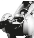
Figure 19 Remove head cap screw
