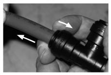
To remove a pipe, push the collar inwards, and then remove the pipe.
