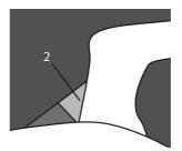
Figure 16 Wear indicator - good condition
