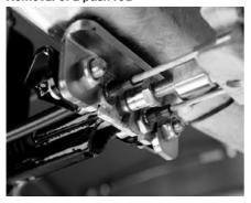
Using a 17mm spanner, slacken locking nut on push rod away from Bowden cable abutment as directed above.
