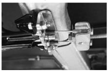
Re-apply the removed locking nut onto brake rod thread to secure ball nut as shown above. ATC is now deactivated.
