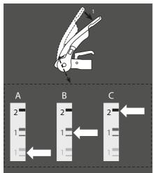
Figure 13 - Checking left / right friction pads
