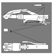
Figure 5 Lubricate/grease the parts indicated.
