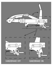
Figure 4 Handbrake lever operation
