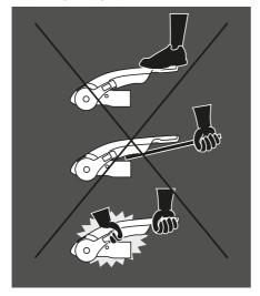
Figure 11 - How not to operate the stabiliser handle
