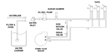
When power is supplied to the pump, it will draw water from the external container through the water inlet mounted on the side of the caravan, and pump it to the caravan taps, shower and water heater.
