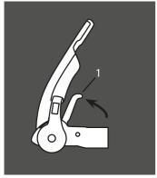
Figure 8 - Pull coupling handle up
