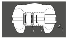
Figure 14 Remove worn pads
