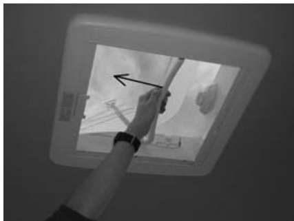
Pull the bar down and forwards (Fig. B).
