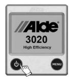
The system will now be drawing variable 0.1–1.5 A of current from the 12v supply.
