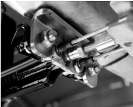
Using a 17mm spanner, slacken locking nut on push rod away from Bowden cable abutment
