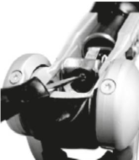
**Fig 4.** Remove head cap screw
